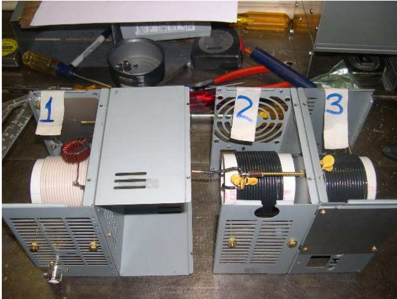
Figure 1: Assembly of the 3 boxes. Note the lead of the coil in box 2 ready to solder through to box 1 when assembled. [ high resolution version ]
