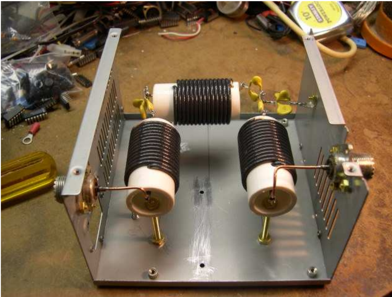
Figure 2: Connector end of case showing coil to input and output connectors. [high resolution version]
