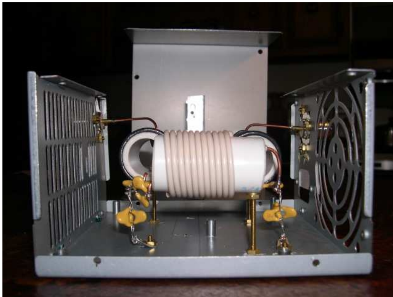
Figure 1: Capacitor wiring and middle coil lead. [ high resolution version ]
