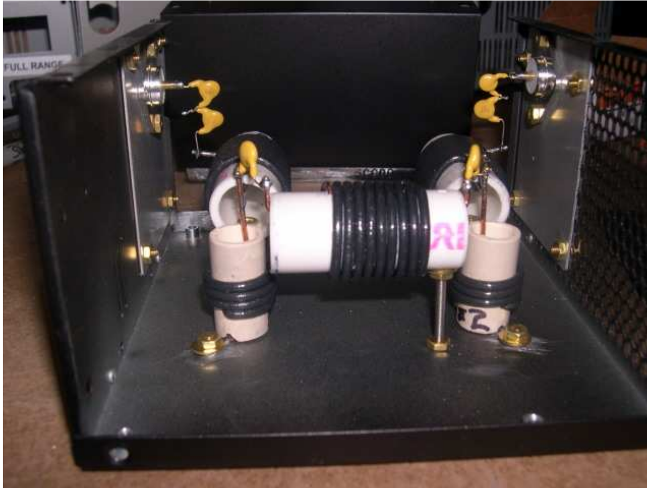
Figure 3: Coil mounting detail. Note the mounting of the shunt coils and the notch to pass the ground lead of coil to the grounding bolt with flat washer and nut. Also the mounting of the series coils on the single bolt. [high resolution version]
