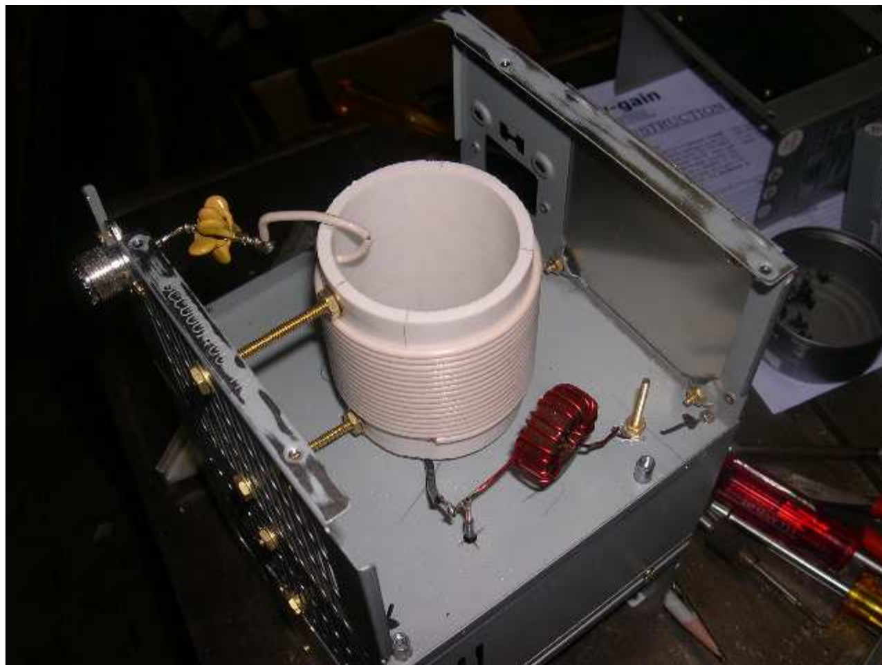
Figure 3: Box 1 coil and capacitor mounting detail. [high resolution version]
