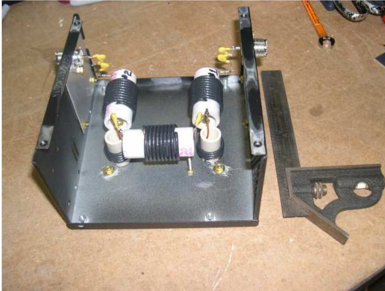
Figure 4: Overall views of filter showing capacitors. [ high resolution version ]
