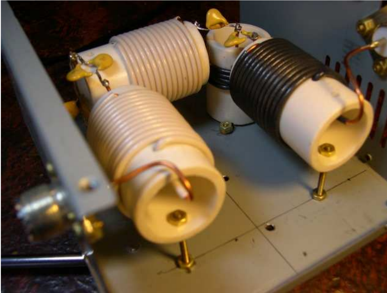
Figure 4: More detail of the capacitor wiring. [ high resolution version ]
