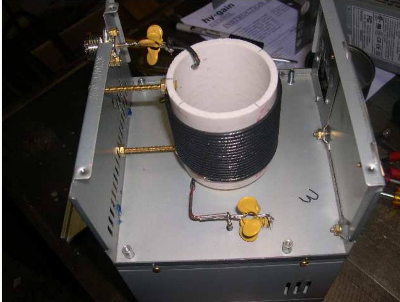
Figure 2: Box 3 coil and capacitor mounting detail. [high resolution version]
