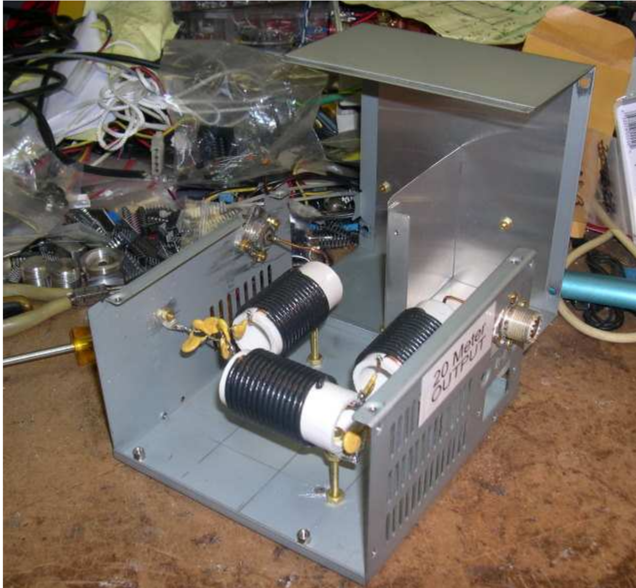
Figure 2: Typical Ugly Filter construction
