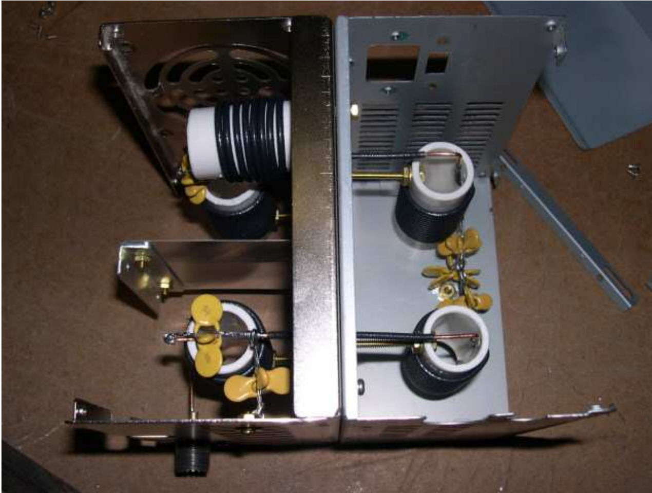
Figure 4: Overall view showing the chassis construction with two PC power supply cases mounted back-to-back. [high resolution version]
