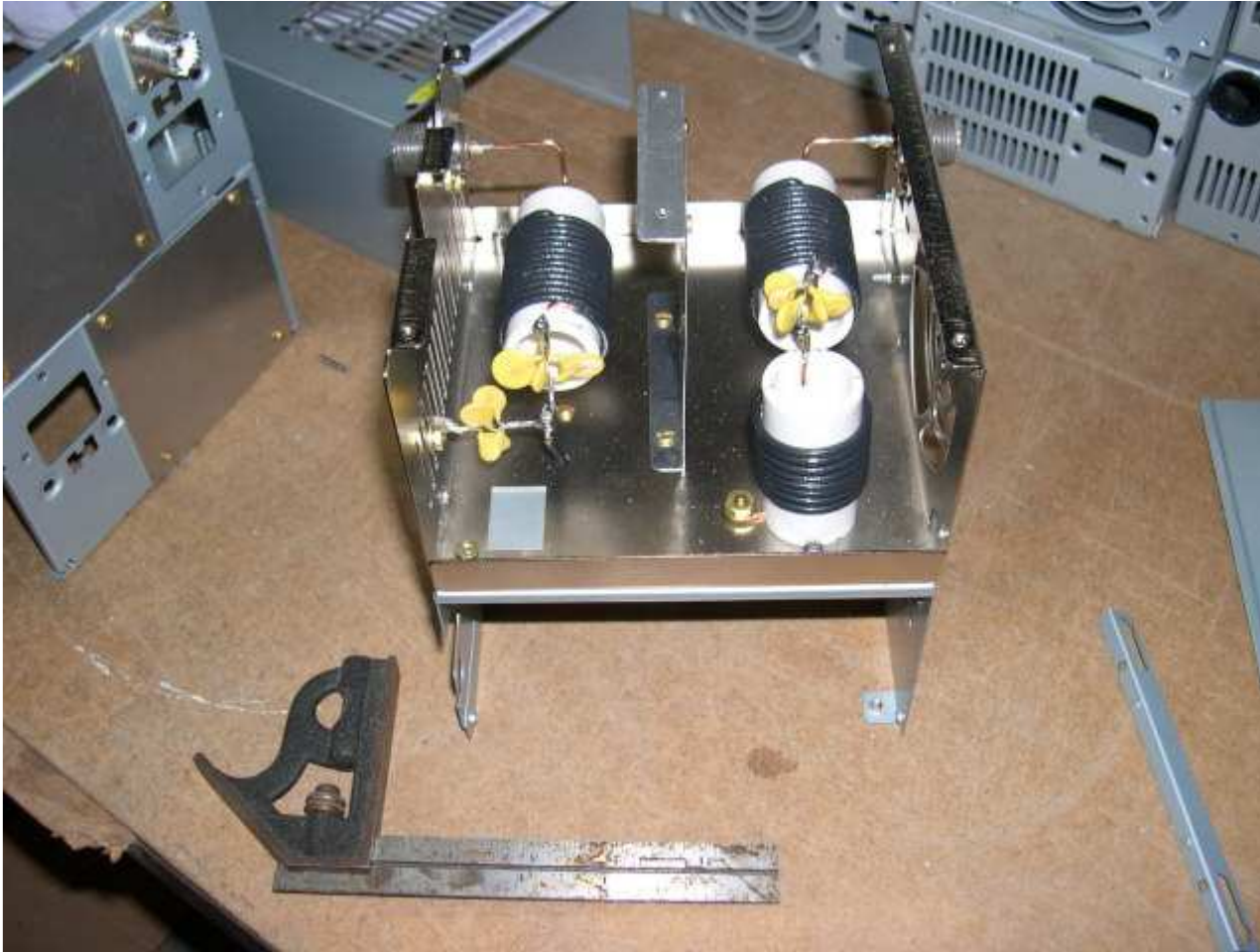
Figure 2: Input/output connector view. This photo shows the input and output connectors and the shunt capacitor and coil. The leads pass thru the center of the case via holes drilled in the case. These feed through wires are insulated with the normal PVC wire insulation. The points in the circuit that are feed through have been chosen to be low voltage points in the circuit so the danger of voltage breakdown is low, but it is advisable to be sure there are no sharp burrs on the holes to puncture the insulation on the wires. [high resolution version]
